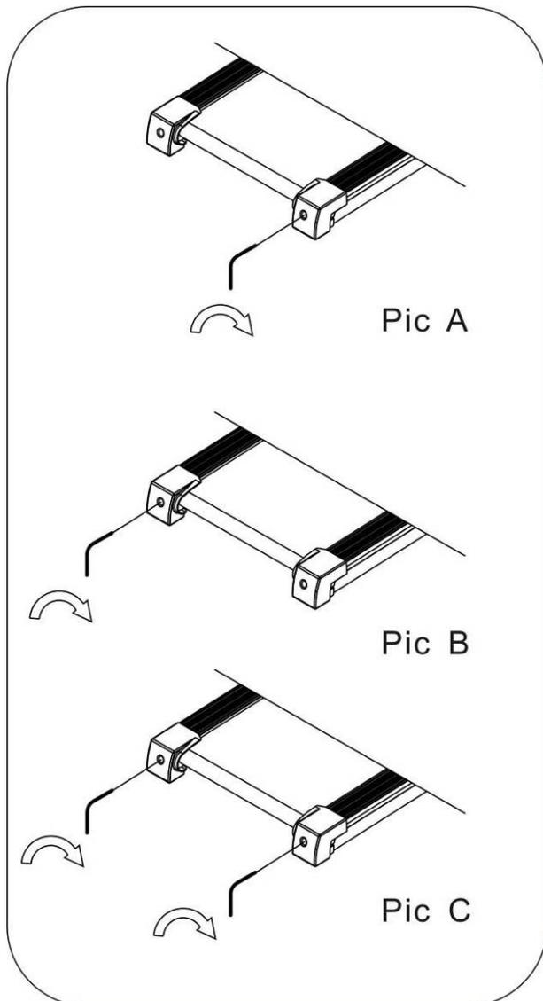
If the belt has drifted to the right, unplug the safety lock and power switch, and turn the right adjusting bolt 1/4 turn clockwise, then insert the power switch and safety lock, make the treadmill running, observe the running belt deviate condition. Repeat above steps until the running belt be placed in the middle. **See picture A**
