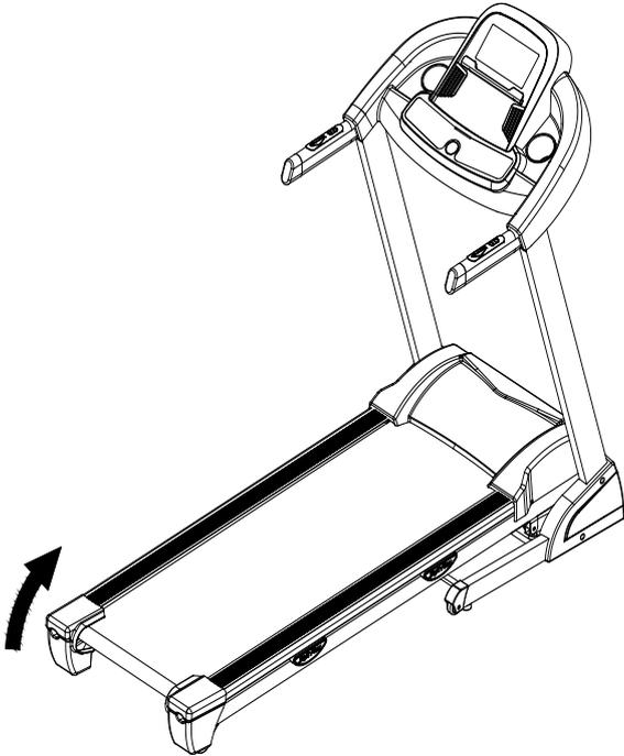
Lift up the machine and force to pull up until you heard "click" that made by safety casing stuck the pneumatic cylinder.
